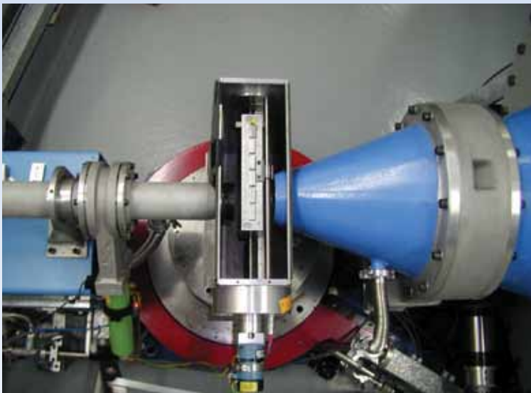
Samples on AUSANS at the HIFAR reactor
