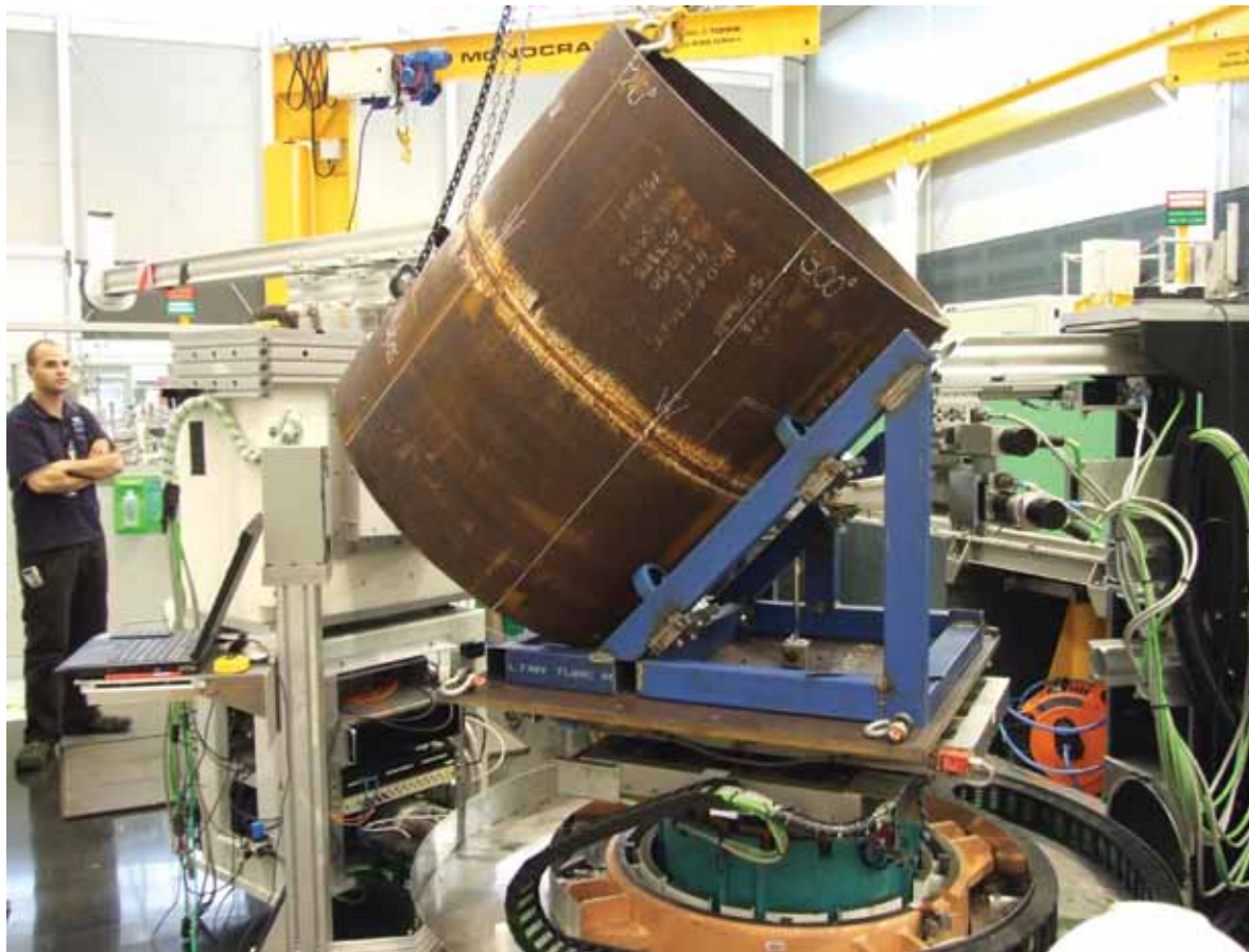
KOWARI (with 640kg sample from the Welding Institute, UK)
