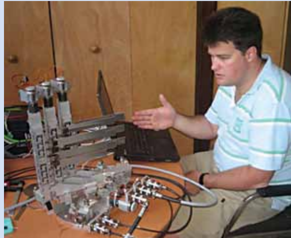
Dan Bartlett and the PELICAN triple monochromator
