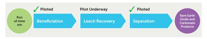
Figure 1: Three stage process developed by Peak for Nqualla's rare earth mineralisation and pilot plant status.
