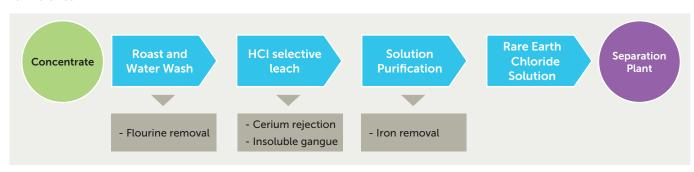
Figure 3: Simplified overview of Peak's Leach Recovery flowsheet being piloted at ANSTO.
