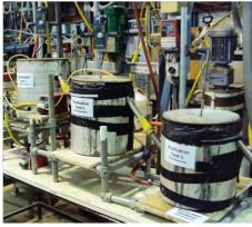
**Figures 4 and 5:** Leach and Purification sections of the Pilot Plant at ANSTO
