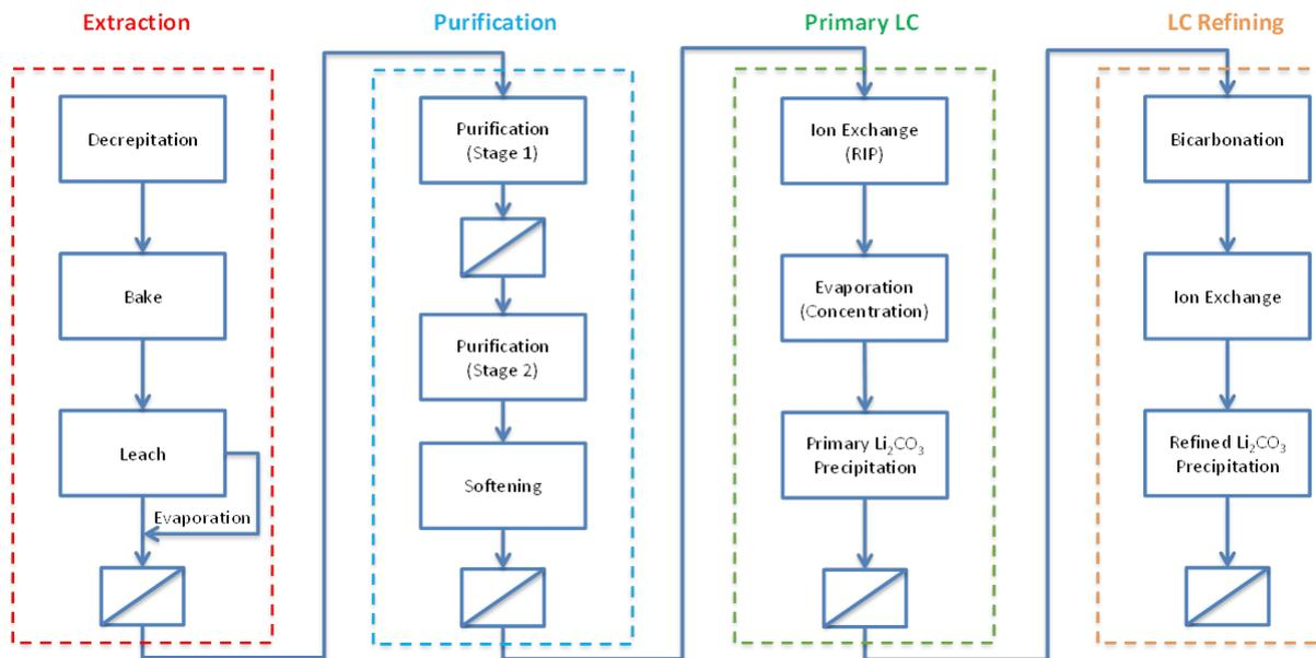
Figure 1: Conventional spodumene processing flowsheet
